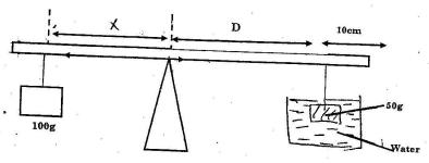
The balance is attained by adjusting the position of the 100g mass. Note that the direction X and D are measured from the knife edge and the 50g mass is fully submerged in the water
