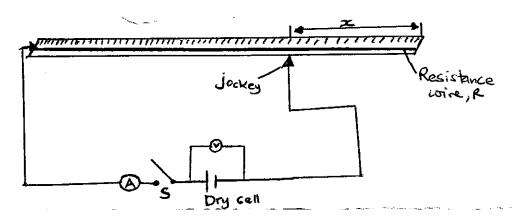
(ii) Adjust the length x of the wire to 25cm by placing the jockey at point A. record the ammeter and voltmeter readings in the table below.
