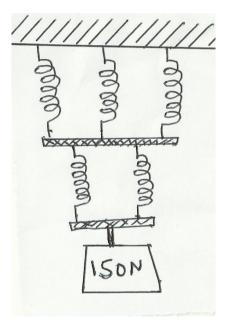
Determine the total extension caused by the 150N weight.
