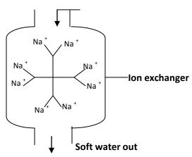
(i) Draw the ion exchanger and show how it will appear at the end of softening process. (2 marks)
