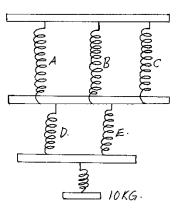
When a mass of 10g was hanged on spring A, its extension was 5cm. Find the extension of thecombination shown if each spring has mass of 50g.(3 marks)
