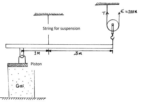
The area of the piston is 10cm<sup>2</sup> and the volume of the gas is 20cm<sup>3</sup>. The weight of the pulley, the beam and the frictional forces at the movable parts are taken to be zero. If the beam is in equilibrium,
